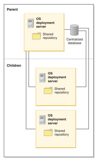
Figure 2. Single database architecture
