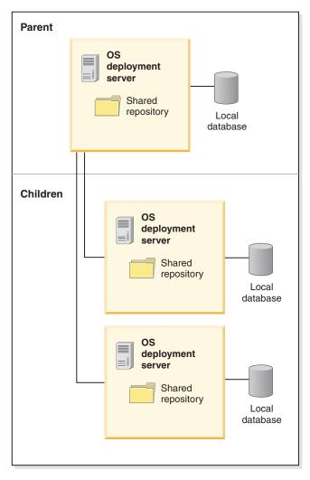
Figure 3. Multiple databases architecture
